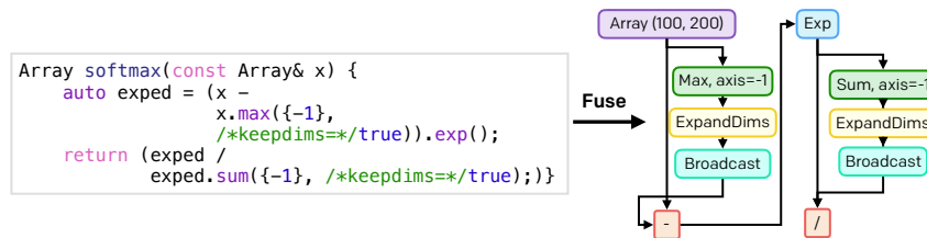
Figure 1: Adjacent operations with the ability to be JIT compiled can be joined into a single compilation unit via Fusion.
